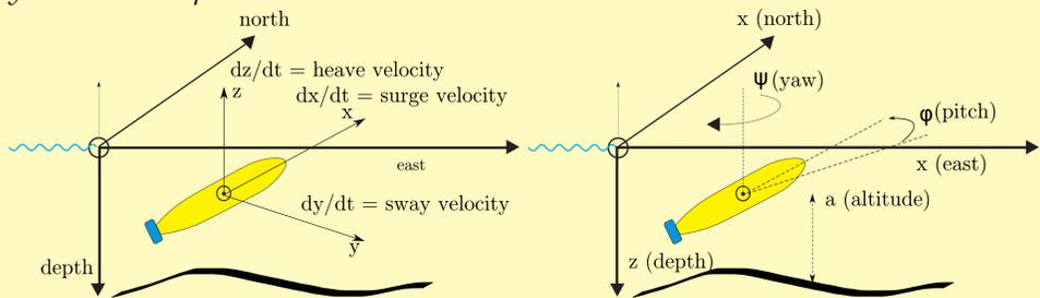
5 d.o.f. system model is describing how the state  $\mathbf{X}(k)$  evolves in time. It is a *constant speed* model [1] that uses previous state  $\mathbf{X}(k-1)$  corrupted with zero-mean GRV acceleration noise to make a prediction of the next state vector value.
