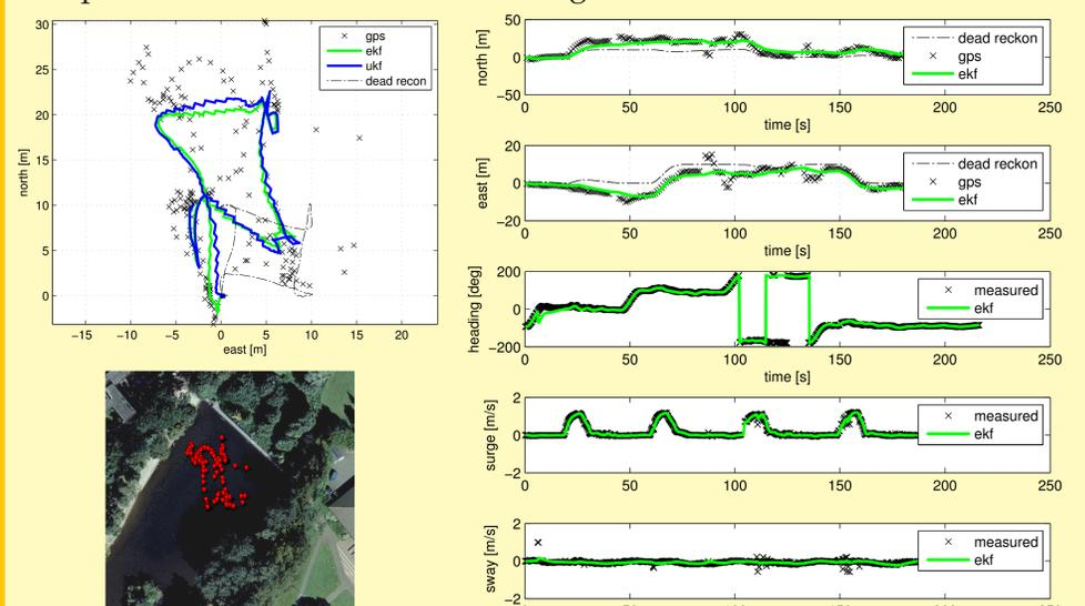
EKF improves the localisation performance, even when confined to blend imprecise and sketchy position data from GPS.
