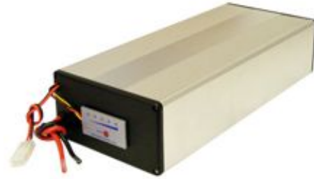
Fig. 5: One of the four battery packs supplying the power to Nessie VI.
